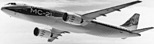
The most innovative feature of MC-21 is the composite wing. TsAGI has performed a large scope of calculations and tests of the static stiffness, life cycle and aero elasticity using both separate samples and full scale structure with the following purpose:
