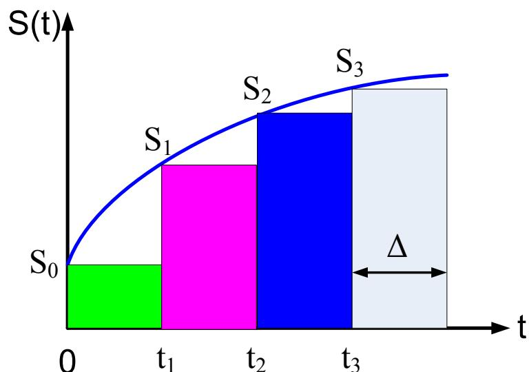
$$\alpha_k(t) = S_k [\sigma(t - t_k) - \sigma(t - t_k - \Delta)]$$
