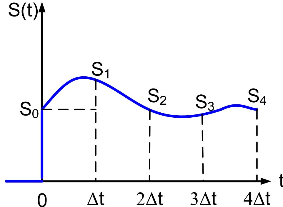
$$S(t) \cong S_0\sigma(t) + (S_1 - S_0)\sigma(t - \Delta t) + (S_2 - S_1)\sigma(t - 2\Delta t) + \dots =$$
